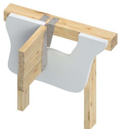
Typical FWHL solid sawn installation (I-Joist similar)
